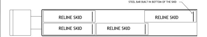
3 REMOVE BAR AND UNLOAD SKID USING FORKLIFT
