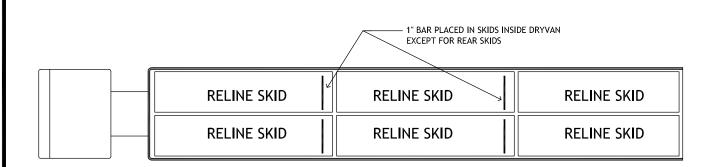
1 REMOVE FIRST ROW OF RELINE SKIDS FROM DRYVAN USING FORKLIFT
