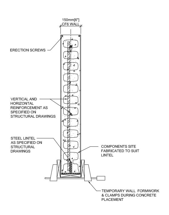
NOTE: SITE FABRICATE COMPONENTS AT EACH SIDE OF OPENING TO INSTALL LINTEL
