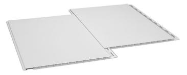
RELINE is available in 12" and 18" wide panels by 3/8" thick, providing a finished face with interlocking joints and fastened at 24" maximum. Trim accessories are available for perimeter conditions, edges of openings and panel joints.
