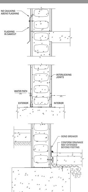
A waterstop placed at the base of the wall will not prevent water rising on the inside of the wall in the gap between the concrete and the PVC and crossing the wall above the waterstop. The water level can rise on the inside of the wall to the height of the hydrostatic head.
