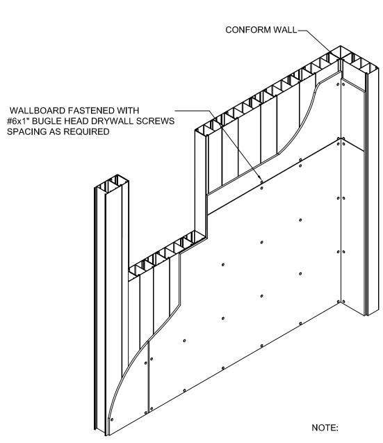
INSTALL SCREWS WHILE CONCRETE IS GREEN OR USE CONCRETE SCREWS IN DRILLED HOLES.
